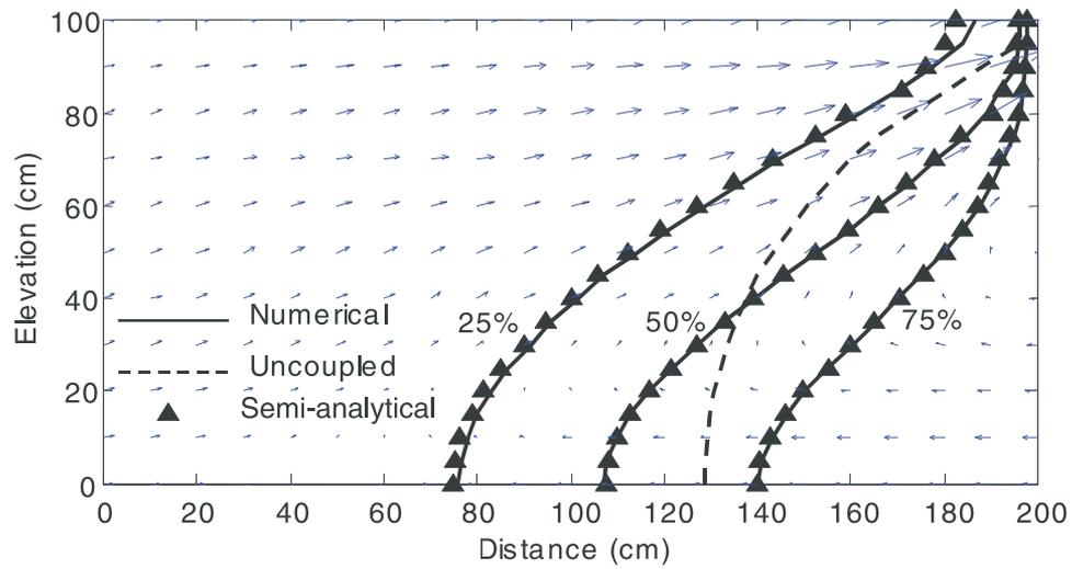
**Figure 3.** Comparison of numerical and semianalytical results for the modified Henry saltwater intrusion problem  $a = 0.1315$ ,  $b = 0.2$ , and  $\xi = 2.0$ . The velocity distribution and uncoupled 50% numerical isochlor (dashed) are also shown.
