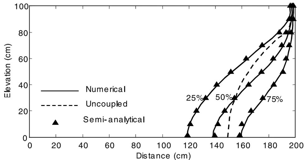
**Figure 2.** Comparison of numerical and semianalytical results for the standard Henry saltwater intrusion problem  $a = 0.263$ ,  $b = 0.1$ , and  $\xi = 2.0$ . The uncoupled 50% numerical isochlor (dashed) is also shown.
