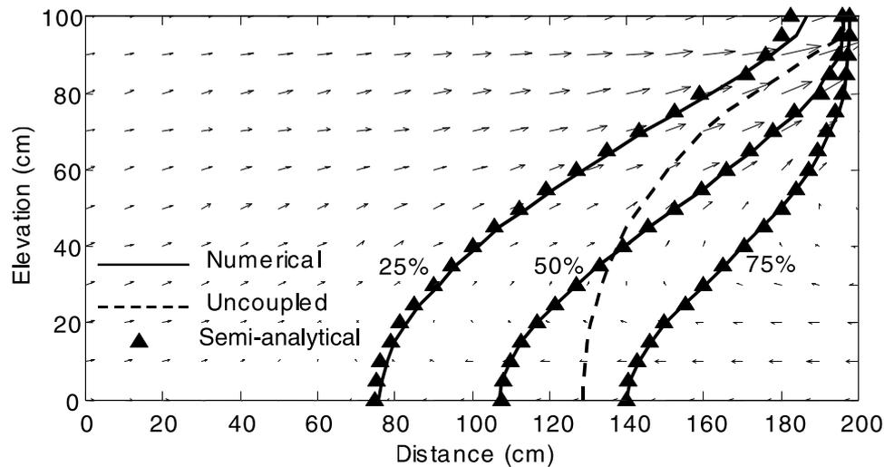
**Figure 3.** Comparison of numerical and semi-analytical results for the modified Henry saltwater intrusion problem  $a = 0.1315$ ,  $b = 0.2$ , and  $\xi = 2.0$ . The velocity distribution and uncoupled 50% numerical isochlor (dashed) are also shown. See color version of this figure at back of this issue.
