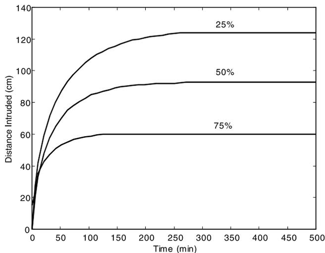
**Figure 4.** Transient position of the intersection of the 25%, 50%, and 75% isochlorers with the base of the aquifer for the modified Henry saltwater intrusion problem  $a = 0.1315$ ,  $b = 0.2$ , and  $\xi = 2.0$ .
