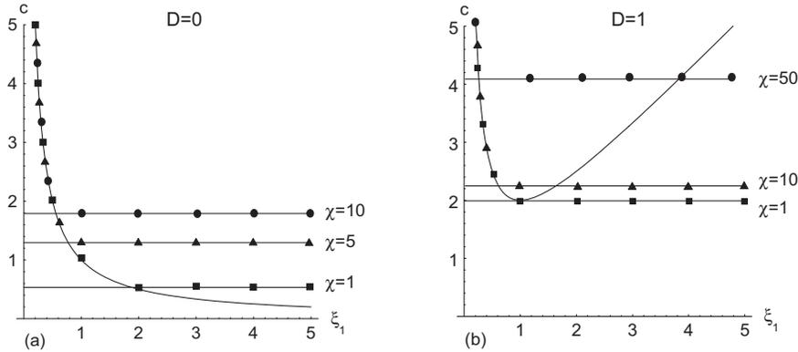
FIG. 4.1. Numerical wave speed  $c$  versus  $\xi_1$  for initial data of the form (4.1)–(4.2). Numerical results are shown in squares, circles, and triangles. These results were generated using  $\Delta x = 0.05$  and  $\Delta t = 0.01$ . The continuous curves are given by (4.7). The horizontal lines represent  $c_{min}$ . Here  $\beta = 1$  and  $\gamma = 1$ . (a) With  $D = 0$  and increasing values of  $\chi$ . (b) With  $D = 1$  and increasing values of  $\chi$ .
