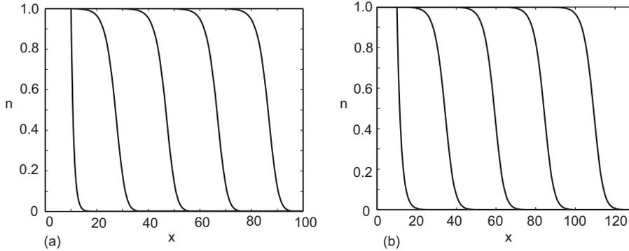
FIG. 6.2. Numerical solutions of  $n(x,t)$  for the Fisher equation with  $D = 1$ ,  $\Delta x = 0.05$ , and  $\Delta t = 0.01$ . (a) Solutions at  $t = 0, 10, 20, 30$ , and  $40$  left to right with  $\xi_1 = 10$ . The computed wave speed is  $c = c_{min} = 2$ . (b) Solutions at  $t = 0, 10, 20, 30$ , and  $40$  left to right with  $\xi_1 = 0.5$ . The computed wave speed is  $c = 2.5$ .
