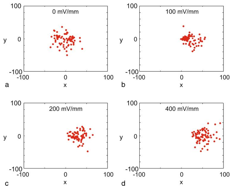
**Fig. 2** End points of cell trajectories under different experimental conditions. Results correspond to: **a**  $EF = 0$ ; **b**  $EF = 100$ ; **c**  $EF = 200$ , and **d**  $EF = 400$  mV/mm. All trajectories are shifted so that the initial location of the trajectory is at the origin. In each subfigure there are 80 red dots, each corresponding to the location of the each cell after a duration of two hours
