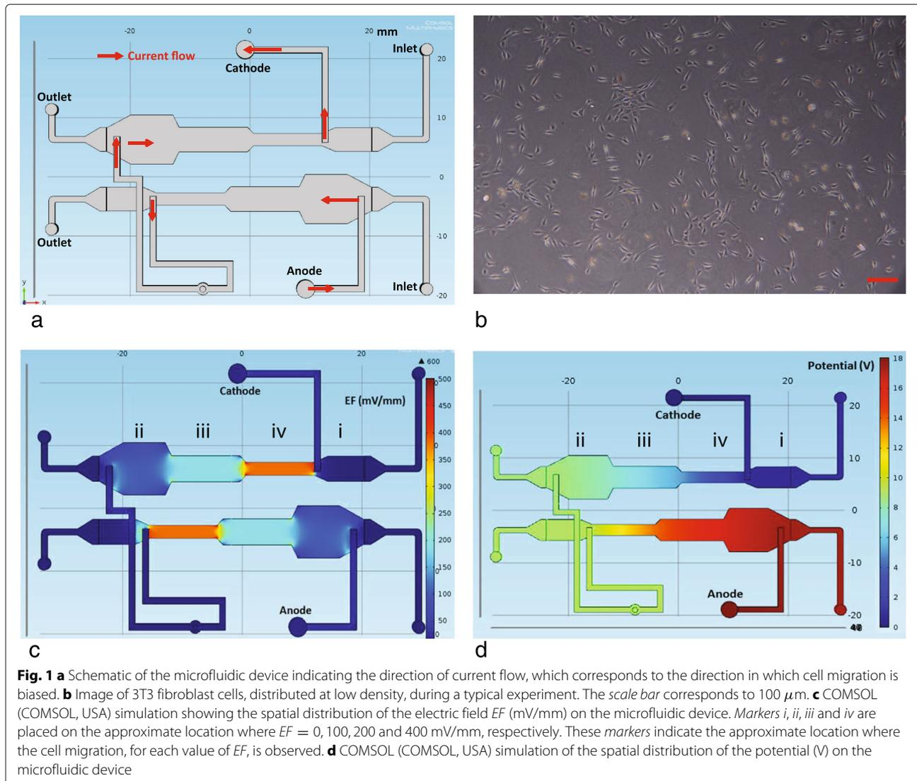
a range of gradients,  $EF = 0, 100, 200$  and  $400$  mV/mm, within the experimental apparatus (Fig. 1a, c-d) are analysed [35]. Since 3T3 fibroblast cells are known to migrate towards the cathode in these types of experiments [35], the Cartesian coordinate axes are aligned so that the positive  $x$ -direction points towards the cathode (Fig. 1c-d). We note that there is no gradient in the  $y$ -direction (Fig. 1c-d).
