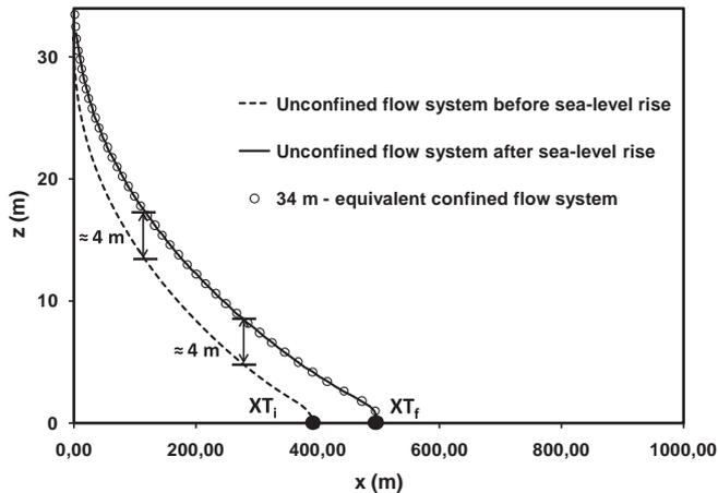
Fig. 8. Comparison of steady-state salt wedges predicted before the sea-level rise in the unconfined system, after the sea-level rise in the unconfined system, and in an equivalent 34-m thick confined-flow system.
