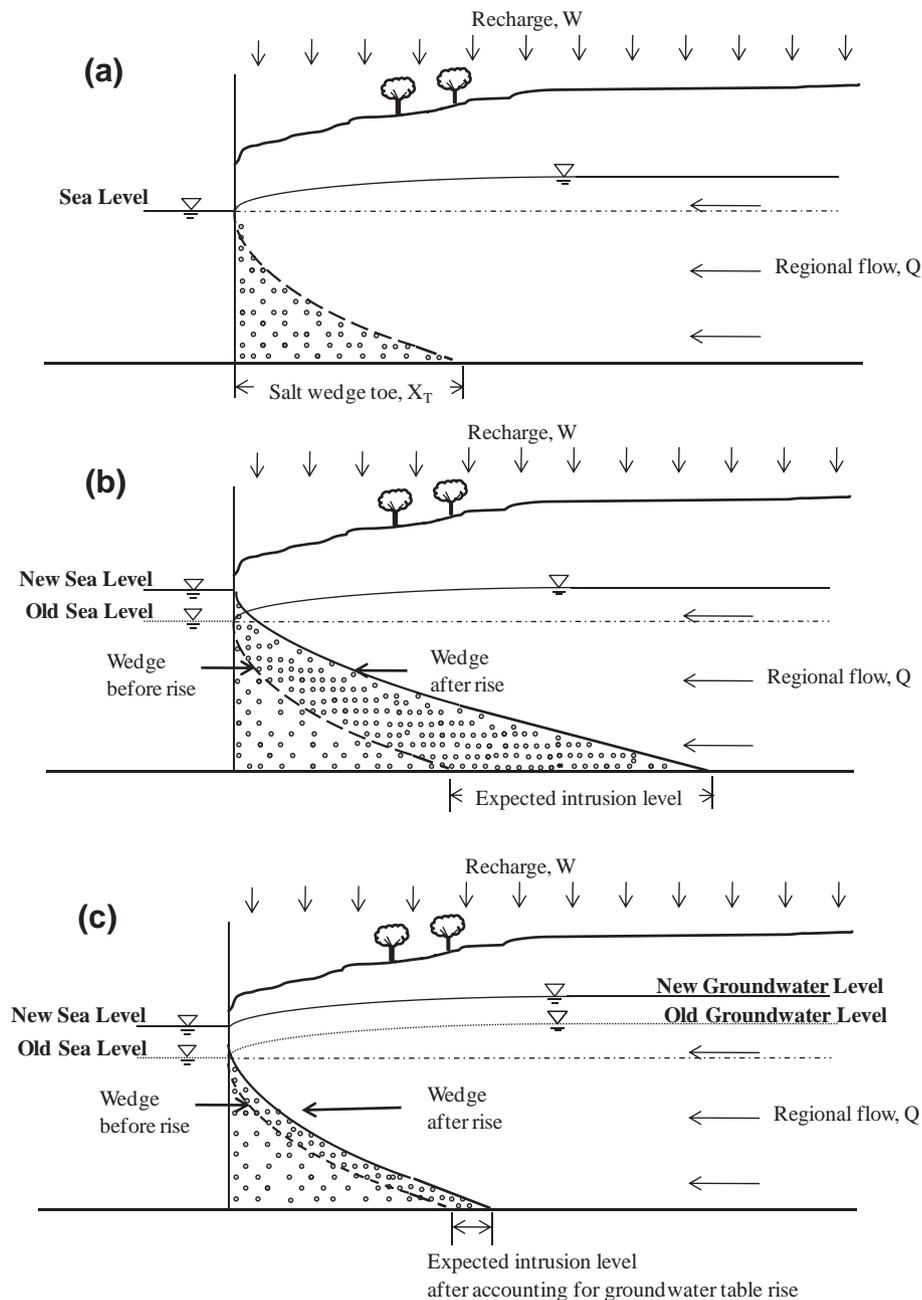
**Fig. 1.** Comparison of conceptual models used for visualizing the impacts of sea-level rise on a saltwater wedge: (a) initial salt wedge before the sea-level rise, (b) salt wedge profile after sea-level rise based on a traditional conceptual model that ignores the lifting effect, and (c) a new conceptual model that includes the lifting effect.
