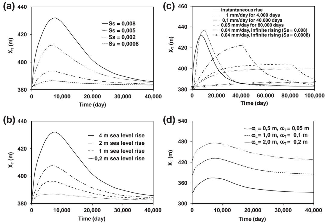
Fig. 5. Sensitivity of the toe position ( $X_T$ ) to (a) specific storage, (b) the magnitude of sea-level rise, (c) the rate of sea-level rise velocity and (d) the dispersivity coefficients.
